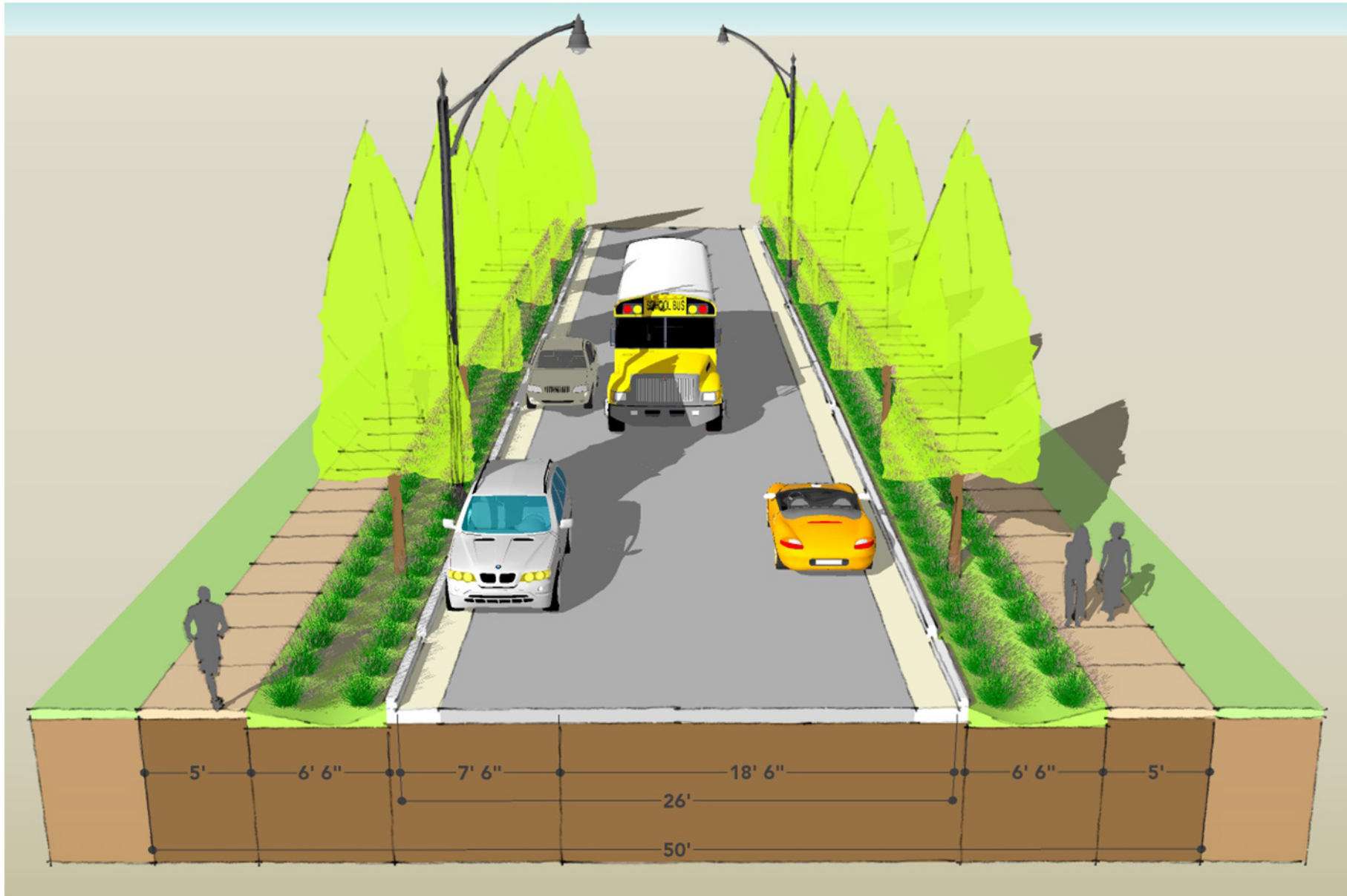
Potential streetscape enhancements to existing 50' ROW includes constructing stormwater bioretention swales in the space between the curb and sidewalk. 5 feet wide sidewalks on both sides of the street allow two pedestrians to walk side by side comfortably. Street trees and decorative light fixtures define the street and help slow traffic.
