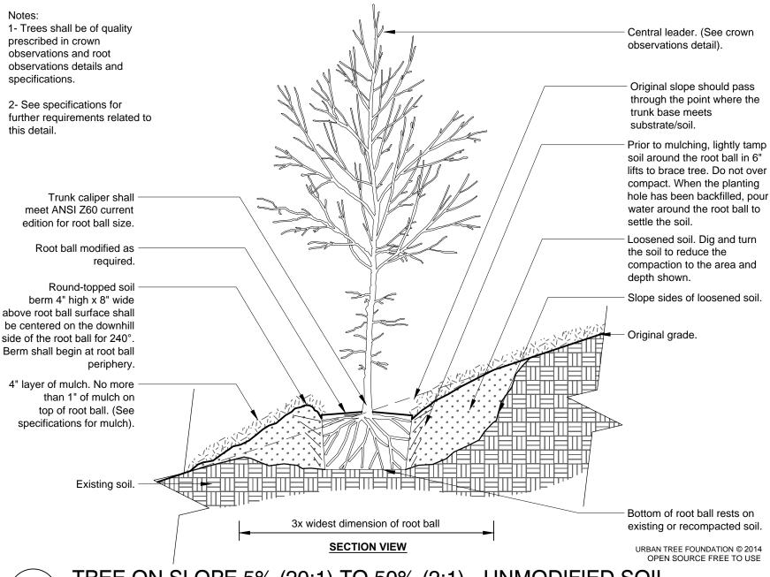
TREE ON SLOPE 5% (20:1) TO 50% (2:1) - UNMODIFIED SOIL
